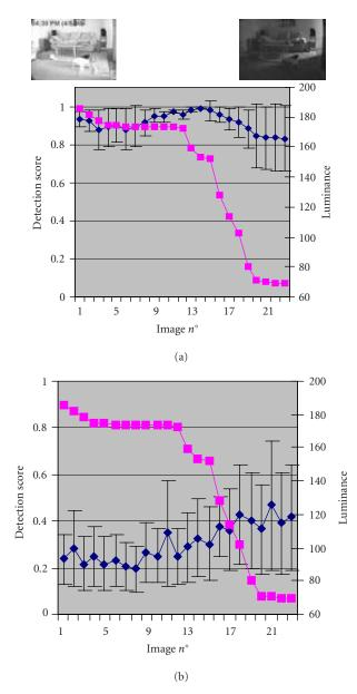
FIGURE 6: Robustness to the variations of illumination. A video sequence with a continuous variation in luminance has been used to follow the detection of homologous interest points from image to image. The figure shows the mean detection score for (a) targets and (b) nontargets superimposed with the luminance curve (expressed in grey levels).
