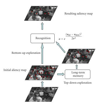
FIGURE 1: An overall presentation of the attentional model. A bottom-up saliency map is biased with the information on the desired target lying in long-term memory.
